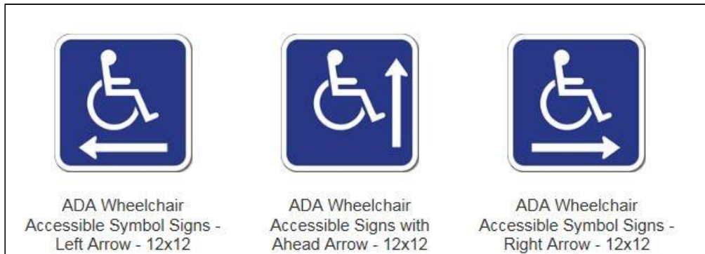
6.0 Item 1(Picture) - Example of compliant directional signage.
